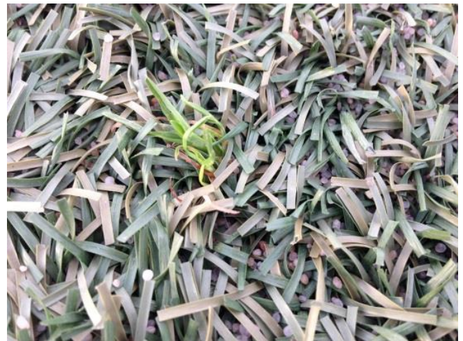
Photo 1: Turf not maintained adequately is showing the yarn is being bent over due to lack of infill and weeds are being allowed to grow
